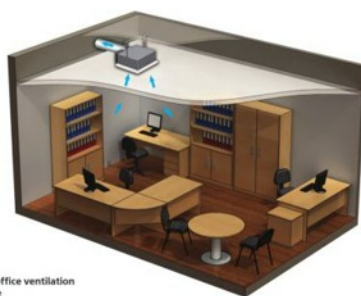
VP fan office ventilation example
